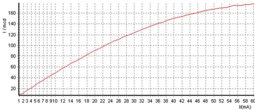
电流-光强曲线 Current-Luminous intensity Curve
