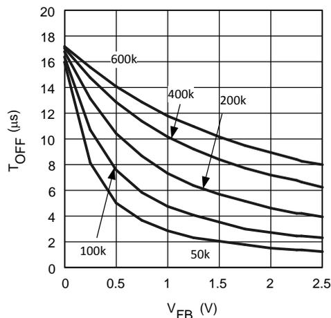
Figure 8. Current Limit  $V_{FB}$  vs  $T_{OFF}$
