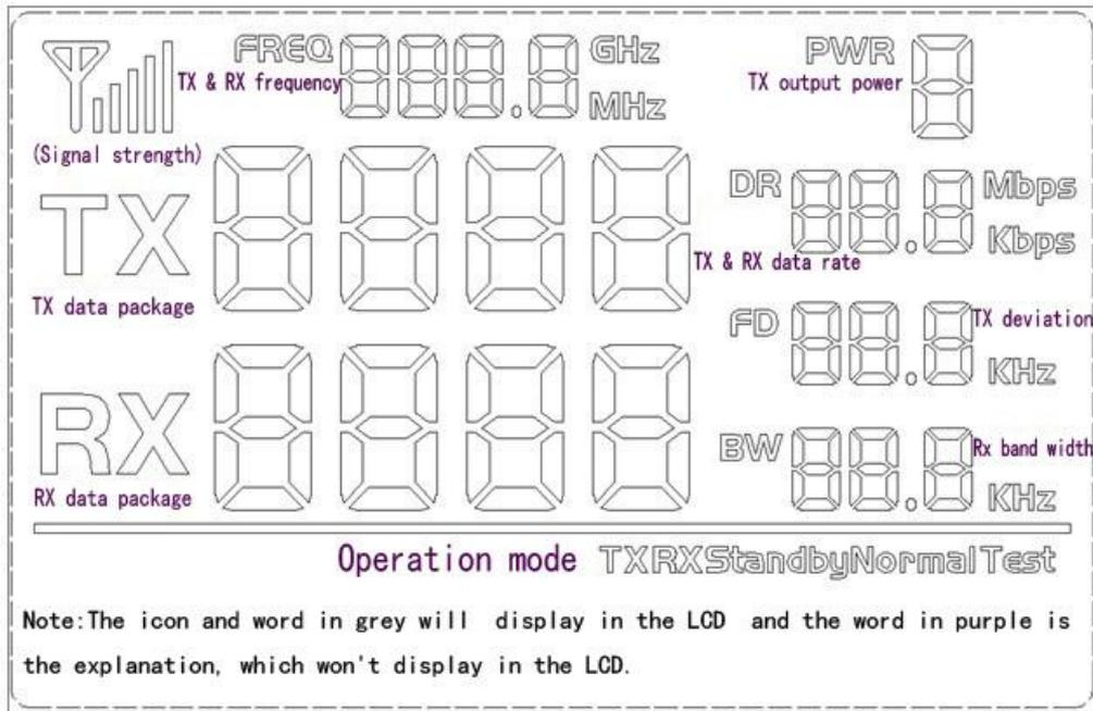
Users can set the parameters of the RF module such as frequency / transmitter power / transmission data rate / working mode through the buttons, and measure the wireless communication distance. Also, all the connection Pins of the module are extended to the demo board, user can use oscilloscope, multi-meter to monitor the operation of the RF module, which is very useful for software programming.
