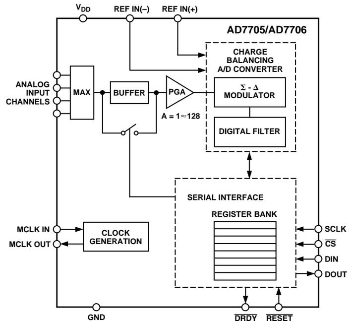
using the input serial port. The part contains self-calibration and system calibration options to eliminate gain and offset errors on the part itself or in the system.
