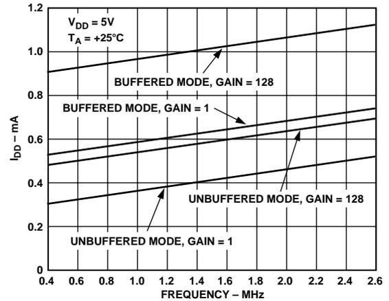
Figure 6. Typical  $I_{DD}$  vs. MCLKIN Frequency @ 5 V
