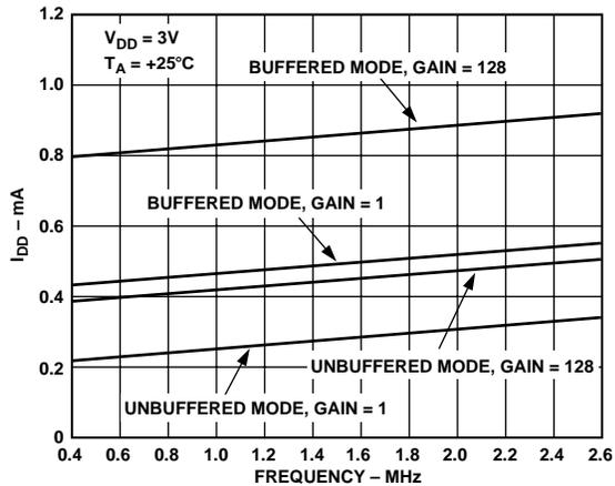
Figure 3. Typical  $I_{DD}$  vs. MCLKIN Frequency @ 3 V
